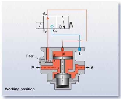
For the "negative" design the pilot valve in rest position is opened and closed in working position.
